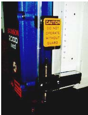
PAT HydroSnubber on Branson 2000 ultrasonic welder
