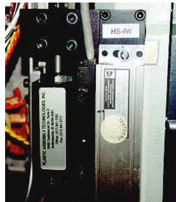
PAT HydroSnubber on Branson 910 IW ultrasonic welder
